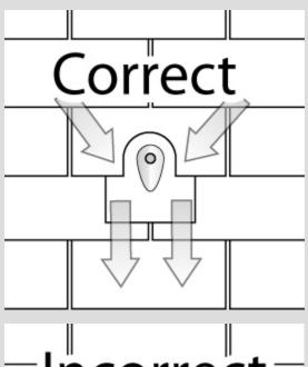
Arrows illustrate the typical water flow on a pitched roof.
