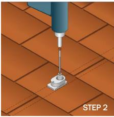
STEP 2: Insert the 5/16" lag bolt and washer through the FastJack® base. Install the lag bolt through the FastJack® using a ½" socket and electric impact wrench.
