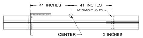
If not using pre-slotted rails, use the 1/2" diameter Irwin™ Uni-Bit® (#10) short nose drill bit to drill U-bolt assembly rail locking holes.
