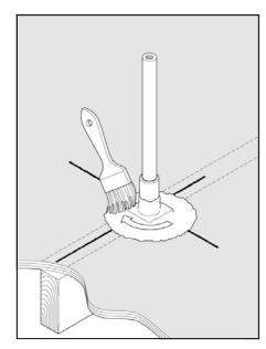
STEP 5: Seal the top of the seal plate with a layer of UV rated seal-ant using a stiff paintbrush. Cover the entire base plate with the seal-ant, at least half the post and about 1-1/2" around the plate.
