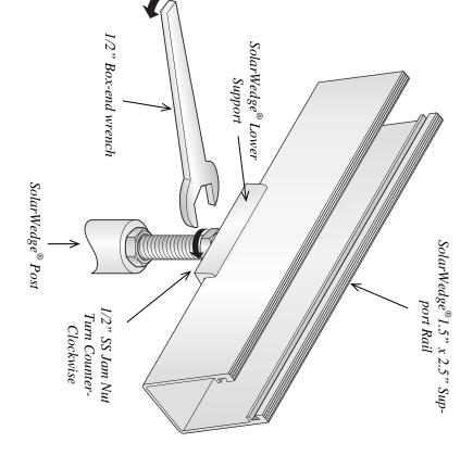
Using a 1/2" Box End wrench, tighten clockwise. Repeat for all attachment the lower jam nut turning counter-
