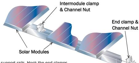
Insert an end clamp at the end of each row of support rails. Hook the end clamps against the long end of the module and square off to the support rail. Tighten the clamps using a 1/2" box wrench or drive socket. DO NOT OVER-TIGHTEN, we recommend a maximum torque of 12 ft. lbs. to prevent damage to the module glass.
