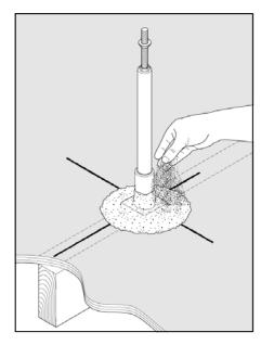
STEP 6: Using Play/Silica sand, cover the sealant. This step prevents debris from sticking to the sealant while drying and gives it a clean, finished appearance. IMPORTANT: Do not install leveling kit hardware until support rail installation.
