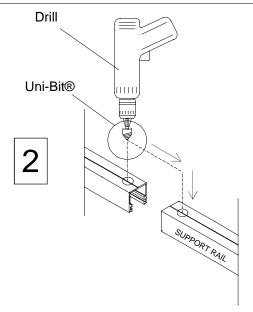
Drill two holes using a 1/2" #10 "Uni-Bit"® - drill at the intersection of the reference mark and the extruded "V" groove in the lower support assembly.
