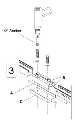
Insert the splice "A" into the channel and install "B" —the two 5/16" bolts / lock washers— into the lower support "C". Tighten using a 1/2" socket. Splice insert is designed to expand into the extrusion walls forcing the rails into alignment, do not over tighten. Roof Trac™ support rails can now can be handled and installed as one solid rail.
