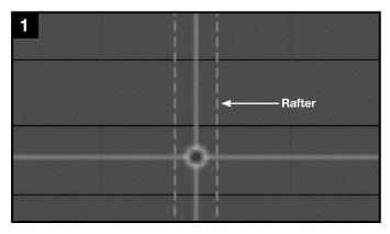
Locate rafters and snap vertical and horizontal lines to mark locations of flashings. Drill 1/4" pilot holes, then backfill with an approved sealant.
