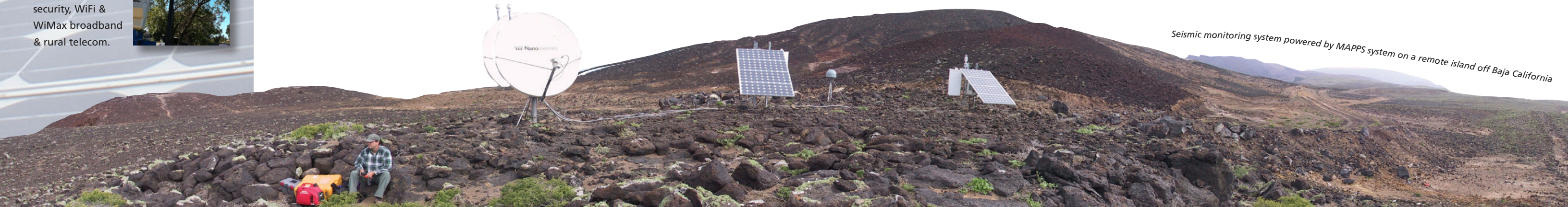
Large battery enclosures for MAPPS solar powered air monitoring system.
