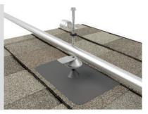
**4**Drive lag into roof decking until secure.
