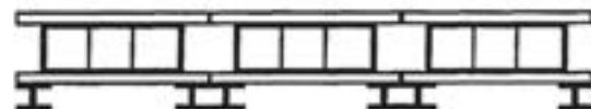
Note: 1) Level modules beneath I-beams in both axes to achieve proper interfacing of channel ends and installation of inter-stack connectors.
