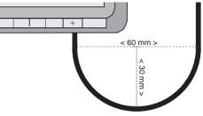
Fig. 7: Minimum bend radius of 30 mm
