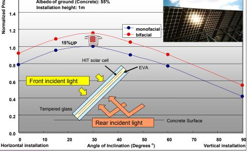
Figure 5. Installation angles and output changes.
