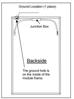
Figure 2. Module Ground Position
