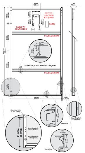
Expanded View of Grounding Holes Frame Cross Section Diagrams
