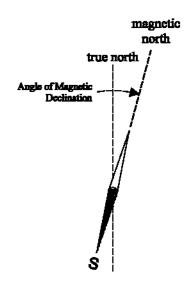
Figure 1 – True South is 12 degrees East of Magnetic South for Phoenix, AZ
