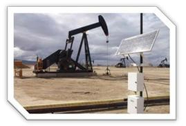
ideally suited for the Oil & Gas industry. In fact, our Class I, Division 2 certified controllers have been proven to reduce the overall cost and time of installation, as they do not require an explosion-proof (purged & pressurized) enclosure.
