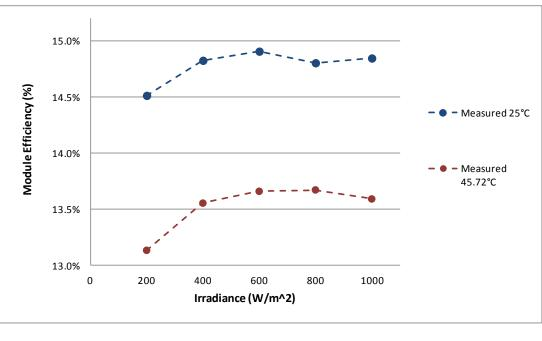
Figure 1 Measured (REC245PE) Efficiency Curves
