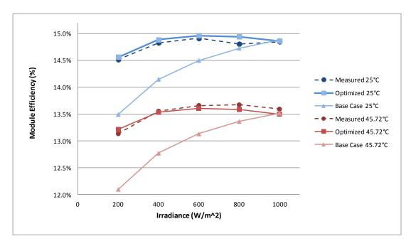
Figure 5 Measured, Base Case and Optimized Efficiency Curves for REC245PE
