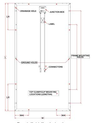
Figure 1: Module Mounting Locations
