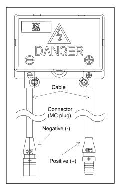
Figure 3: Configuration of Junction Box
