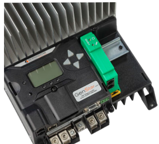
ReadyBMS installed in a GenStar MPPT charger
