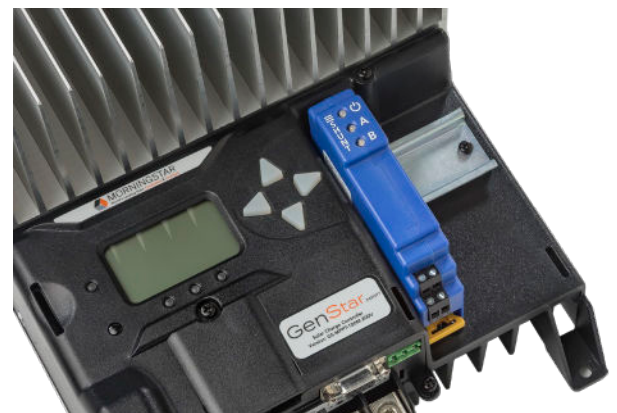
ReadyShunt installed in a GenStar MPPT charger
